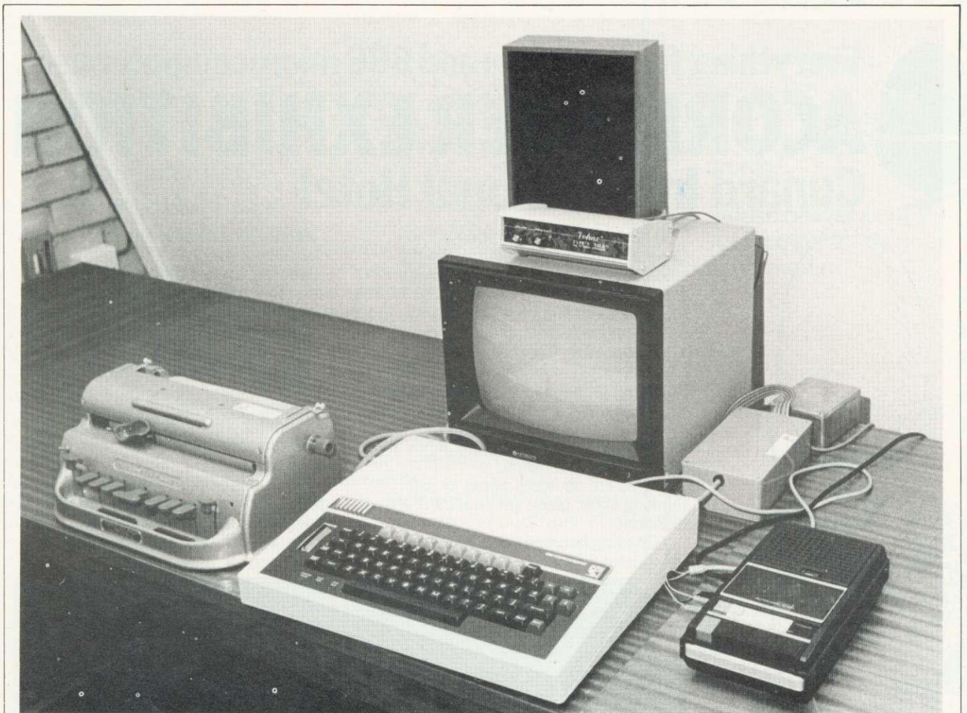
BBC micro flanked by Perkins Braille, with Votrax on top of the monitor
